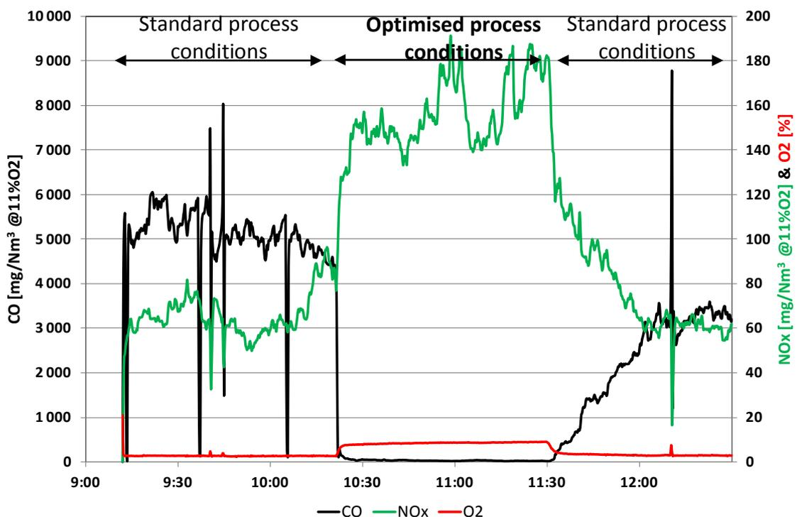
Figure 1: kiln emissions in standard and optimised process conditions
